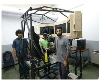
experience for the driver. Kinematic & software systems were explored in the design to synchronise platform movement to improve realism. Safety features were added and modifications were made to improve comfort.
